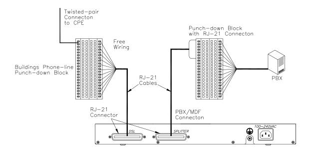
Figure 4-6. Connecting to the Punch-down Blocks
